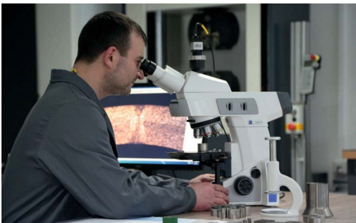
🔍 Every weld, every surface, every structure is inspected in detail. Using high-resolution microscopes or the patented visual seam scanner, Hartmann identifies micro-defects down to six micrometres — setting new standards in non-destructive testing for stainless steel tubes.
