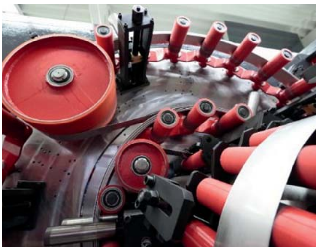
➤ The modern machinery at Hartmann Edelstahlrohre GmbH enables continuous production without downtime thanks to fully automatic strip storage systems.
